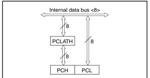
FIGURE 6-12: PROGRAM COUNTER USING THE CALL AND GOTO INSTRUCTIONS
