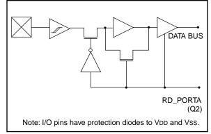
FIGURE 9-2: RA2 AND RA3 BLOCK DIAGRAM
