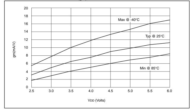
FIGURE 18-6: TRANSCONDUCTANCE (gm) OF XT OSCILLATOR vs. VDD
