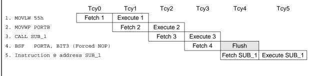
All instructions are single cycle, except for any program branches. These take two cycles since the fetch instruction is "flushed" from the pipeline while the new instruction is being fetched and then executed.
