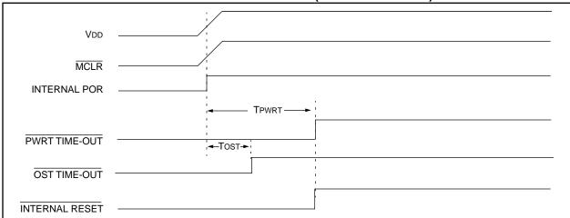
FIGURE 4-2: TIME-OUT SEQUENCE ON POWER-UP (MCLR TIED TO VDD)
