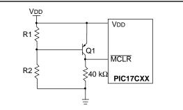
This brown-out circuit is less expensive, albeit less accurate. Transistor Q1 turns off when VDD is below a certain level such that:
