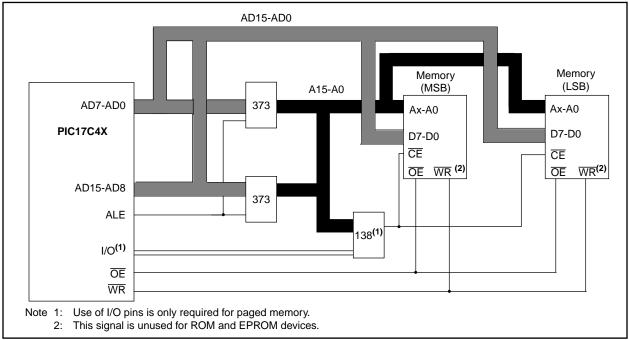
FIGURE 6-4: TYPICAL EXTERNAL PROGRAM MEMORY CONNECTION DIAGRAM
