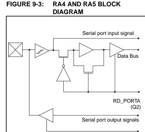
$\overline{OE}$  = SPEN,SYNC,TXEN,  $\overline{CREN}$ ,  $\overline{SREN}$  for RA4  $\overline{OE}$  = SPEN ( $\overline{SYNC}$ +SYNC, $\overline{CSRC}$ ) for RA5
