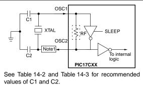
Note 1: A series resistor may be required for AT strip cut crystals.
