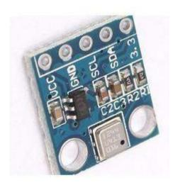
Measuring the absolute pressure of the environment using a digital barometer such as this has some interesting applications. By converting the pressure measured into altitude, you have a reliable sensor for determining the height of your robot, plane.
