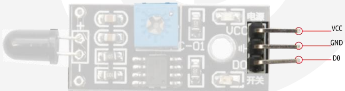
Figure 1 - Flame sensor pin layout
