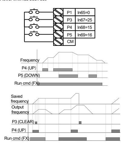
When the Ad66 code is set to 1: The motor accelerates by as much as the step frequency set by the Ad67 code at the multi-function input's positive edge that has been set as the Up terminal signal. The motor decelerates by as much as the step frequency set at the Ad67
