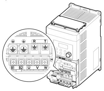
4 Connect the other ends of the ground cables to the supply earth (ground) terminal.
