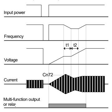
If an instantaneous power interruption occurs and the input power is disconnected, the inverter generates a low voltage trip and blocks the output.
