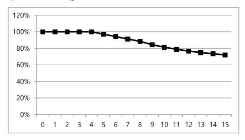
The 0.1 kW–0.2 kW products can be operated at a maximum of 50  $^{\circ}$ C. However, the lifespan of the product may be reduced when operating continuously with a full load when the ambient temperature exceeds 40  $^{\circ}$ C (35  $^{\circ}$ C when an optional vent cover is installed).
