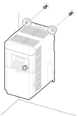
3 Mount the inverter on the wall or inside a panel using the two upper bolts, and then fully tighten the mounting bolts. Ensure that the inverter is placed flat on the mounting surface, and that the installation surface can securely support the weight of the inverter.
