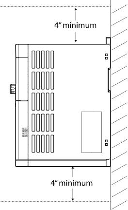
• Ensure sufficient air circulation is provided around the inverter when it is installed. If the inverter is to be installed inside a panel, enclosure, or cabinet rack, carefully consider the position of the inverter's cooling fan and the ventilation louver. The cooling fan must be positioned to efficiently transfer the heat generated by the operation of the inverter.
