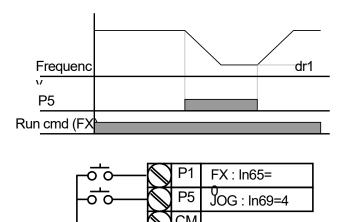
The jog operation is the second highest priority operation, after the dwell operation. If a jog operation is requested while operating the multi-step, up-down, or 3-wire operation modes, the jog operation overrides all other operation modes. The diagram above shows the example when the multi-function input is set to the NPN mode.
