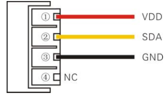
PIC1: AM2305 Pin Assignment
